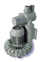
Blower Housing and open/closed impellers made of cast aluminum, Direct motor, IE2-compliant, Integrated silencer, Compact construction, Corrosion-resistant.
